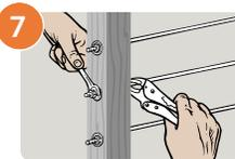
7 Tighten Washer Nuts until you can't flex the cables more than 4 inches apart using your thumb and fingers on one hand. Hold the Threaded Terminal shaft with Vise-Grip pliers while tightening.
