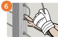
6 Hold the Quick-Connect®SS fitting with one hand and pull the cable tight with the other. The fitting automatically locks when you release the cable.
