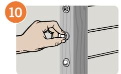
10 Snap on end caps over the exposed Quick-Connect®SS fittings and the Washer Nuts. You're done.
