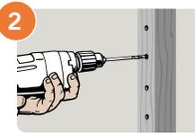
2 Drill holes in posts. Hole diameter depends on assembly size and type of fitting.
