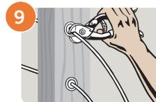
9 Use cable cutters or cut-off disk to trim the excess cable. Grind flush the exposed cable ends with an electric grinder.
